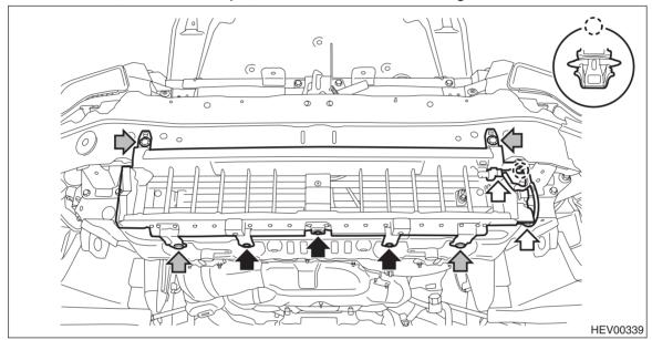
(3) Release the claws and then remove the ambient sensor.
